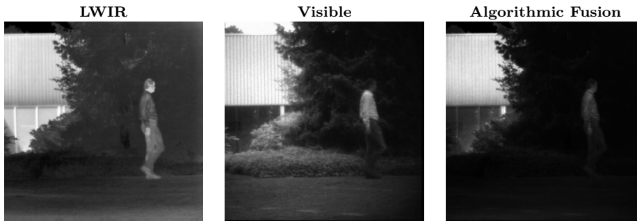
Fig. 4 Examples of LWIR, visible, and algorithmically fused images used for the facing discrimination stimuli. In Experiment 1, white noise was added similar to Figure 3.
